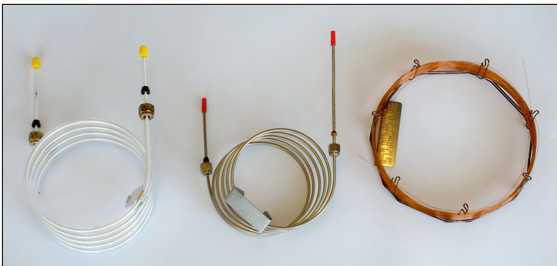
19 20 21 Figure 2.11 A 1/4-inch Glass Packed GC Column, a 1/8-inch Stainless Steel 22 GC, and a Fused Silica Capillary Column (from left to right). 23
