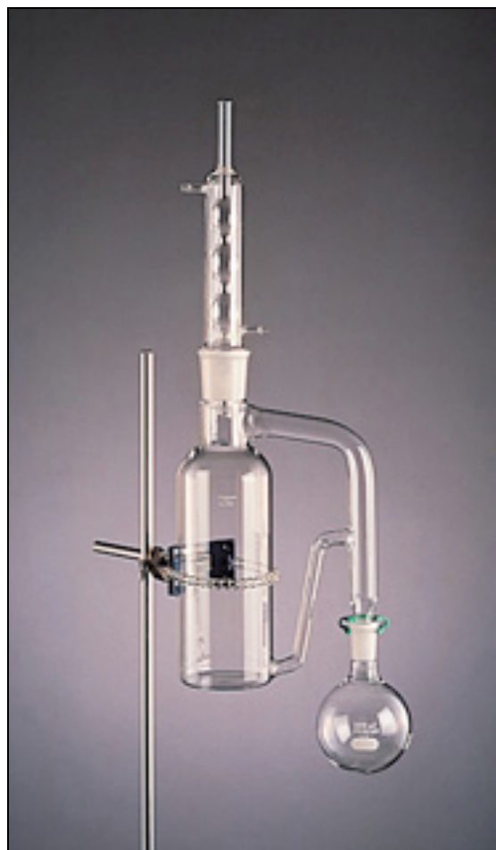
Figure 2.1 A Liquid-Liquid Extractor for Extracting Analytes from Water Samples. Reprinted with permission from VWR Scientific Products International, Chemglass Life Sciences, and Corning.
