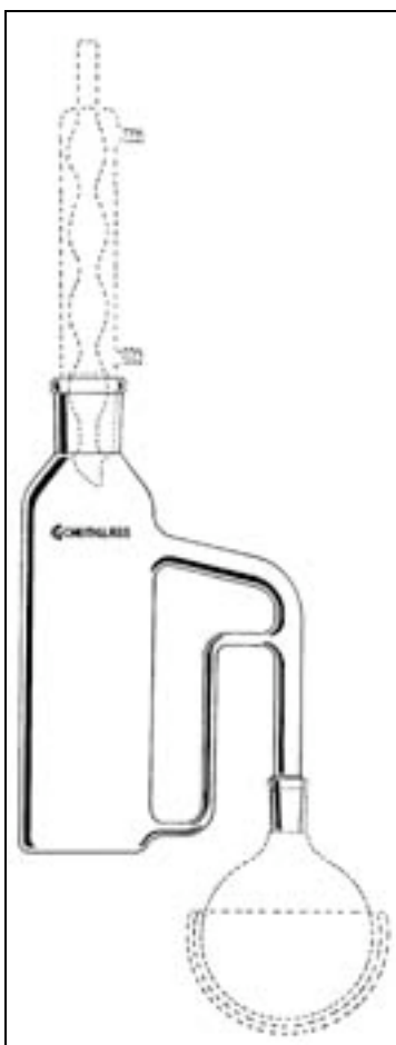
Figure 2.1 A Liquid-Liquid Extractor for Extracting Analytes from Water Samples. Reprinted with permission from VWR Scientific Products International, Chemglass Life Sciences, and Corning.
