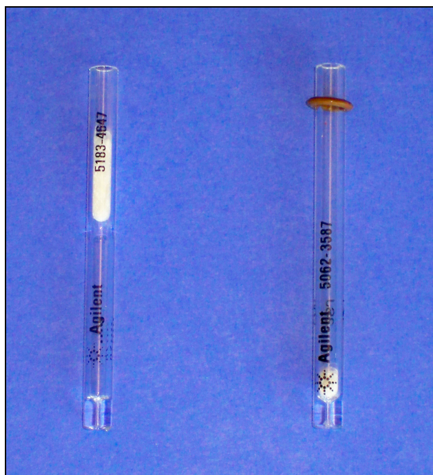
Figure 2.7 Injection Glass Inserts. The insert on the right shows the o-ring that seals the injection chamber and forces carrier gas through the column.
