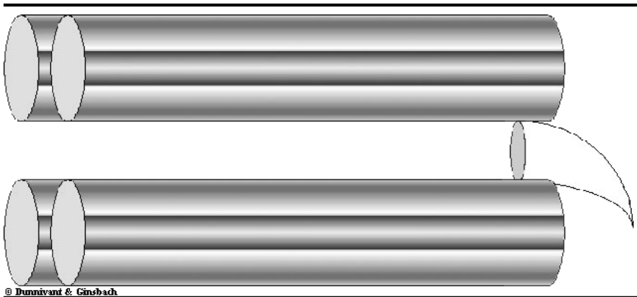
Animation 5.6. Illustration of a Quadrupole Mass Filter.
