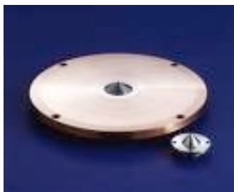
Figure 4-2. Photograph of a Sampler (the larger one) and a Skimmer Cone for ICP-MS.
