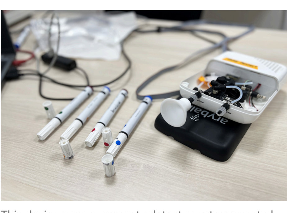
This device uses a sensor to detect scents presented on odor sticks and then sends an electric signal into a participant’s nose. MOUSTAFA BENSAFI
