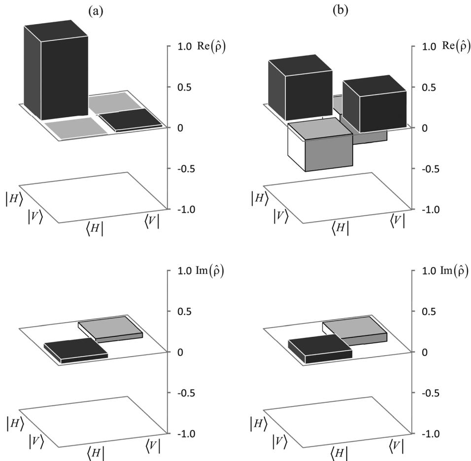
Fig. 5. The real and imaginary parts of the density matrix for the signal beam, with source photons prepared in the entangled state  $|\phi^+\rangle$ . The measurements were conditioned on idler photons detected to be: (a) horizontally polarized at A, (b) linearly polarized along  $-45^\circ$  at A. Dark boxes correspond to positive values while light boxes correspond to negative values.
