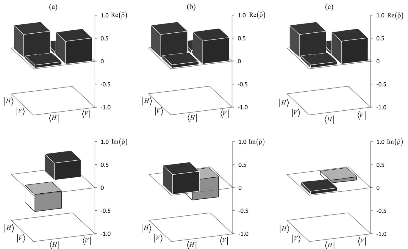
Fig. 4. The real and imaginary parts of the density matrix for the signal beam, with source photons prepared in the entangled state  $|\phi^+\rangle$ . The measurements were conditioned on idler photons detected to be: (a) left-circularly polarized at  $A$ , (b) right-circularly polarized at  $A'$ , (c) present at either  $A$  or  $A'$ . Dark boxes correspond to positive values, while light boxes correspond to negative values.
