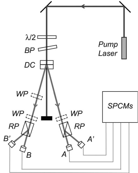
Fig. 2. A schematic of the experimental apparatus. Here  $\lambda/2$  denotes a half-wave plate,  $BP$  denotes a birefringent plate,  $DC$  denotes the down-conversion crystals,  $WP$  denotes an optional wave plate, and  $RP$  denotes a Rochon polarizer. Lenses at  $A, A', B$  and  $B'$  focus the down-converted beams into multimode optical fibers, which direct the light to single photon counting modules (SPCMs).
