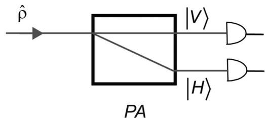
Fig. 1. A polarization analyzer ( $PA$ ) that splits a beam into its horizontal and vertical components.
