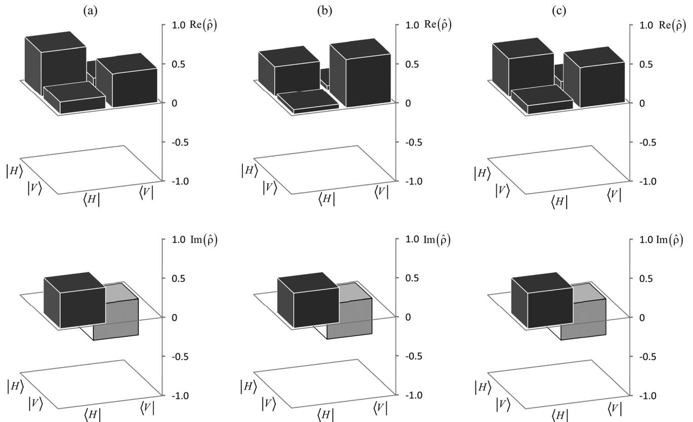
Fig. 3. The real and imaginary parts of the density matrix for the signal beam prepared in state  $|L\rangle_s$ . The measurements were conditioned on idler photons detected to be: (a) left-circularly polarized at  $A$ , (b) right-circularly polarized at  $A'$ , (c) present at either  $A$  or  $A'$ . Dark boxes correspond to positive values while light boxes correspond to negative values.
