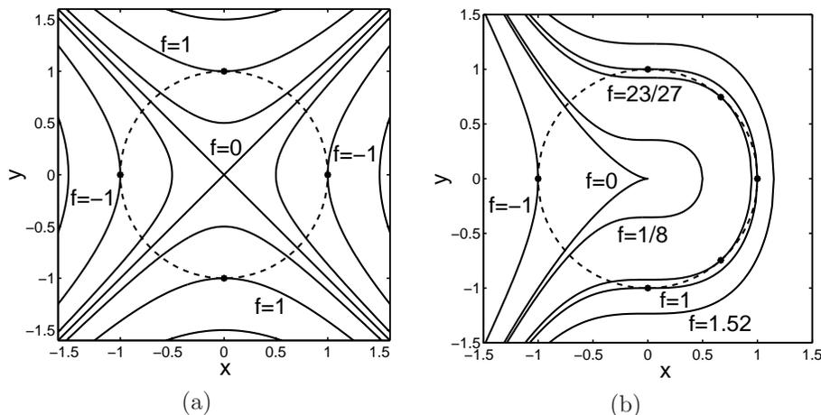
**FIGURE 4.2:** Unit circle  $x^2 + y^2 = 1$  (dashed) and level contours of (a):  $f(x, y) = x^2 - y^2$ , (b):  $f(x, y) = x^3 + y^2$ . The points of tangency are the extreme points of  $f(x, y)$  restricted to the unit circle.
