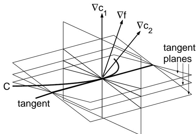
**FIGURE 4.4:** At a solution point of a three-variable optimization problem with two constraints the tangent plane of the level surface of  $f$  and the tangent planes of the two intersecting constraint surfaces  $c_1 = 0$  and  $c_2 = 0$  intersect in the tangent of the constraint curve  $C$ . As a consequence all three gradients are in the normal plane of  $C$  and so are linearly dependent.
