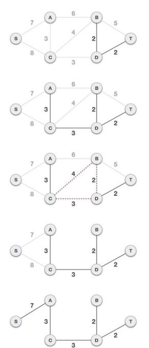
Step 1: Find the arc with the minimum value, and include it in the spanning tree. In this case, we have two arcs with the lowest, and including them both does not create a loop.
