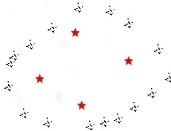
Figure 8.2: If the data lies on a curved surface, then using the mean may pull the centers (stars in the graph) out of the data.
